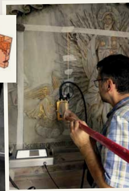
Ground penetrating radar prospection of the Holy Aedicule of the Holy Sepulchre in order to reveal its internal structural layers
