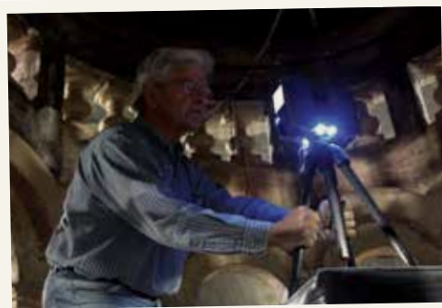
NTUA Prof. Andreas Georgopoulos: Geometric documentation of the inner cupola of the Holy Aedicule, through laser scanning
